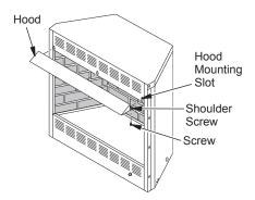
Figure 15 - Installing Fireplace Hood
